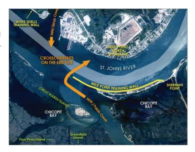
FIGURE 2A: PRE-CONSTRUCTION CONDITIONS AT MILE POINT, LOCATED AT THE INTERSECTION OF THE ST. JOHNS RIVER AND ATLANTIC INTRACOASTAL WATERWAY IN DUVAL COUNTY, FL. NOTE EBB TIDAL CURRENTS INDICATED BY ORANGE ARROWS, PRE-CONSTRUCTION LOCATION OF MILE POINT TRAINING WALL, AND HABITAT LOSS AT GREAT MARSH ISLAND.
