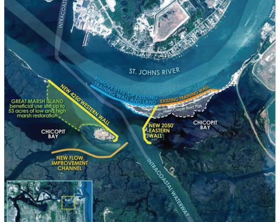
FIGURE 2B: MAP HIGHLIGHTING COMPONENTS (MODIFICATION OF EXISTING WALLS, CONSTRUCTION OF NEW WALLS, ENHANCEMENT OF GREAT MARSH ISLAND) OF THE MILE POINT NAVIGATION PROJECT.
